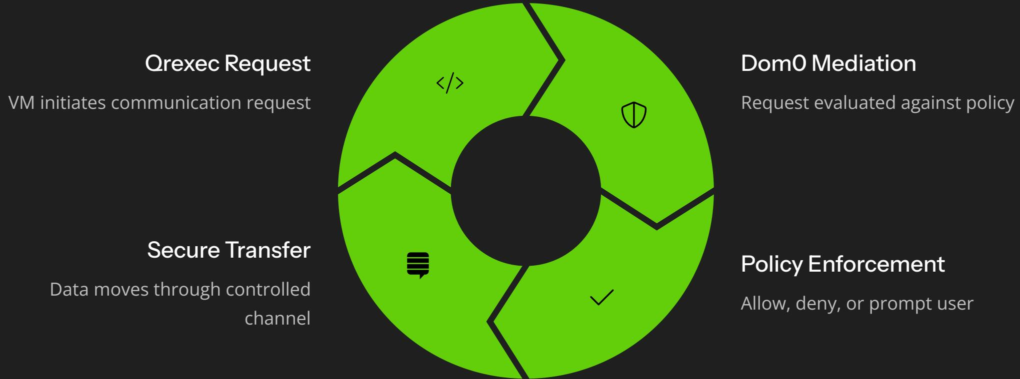
Complete isolation is secure but impractical – qubes often need to communicate in limited ways. The qrexec framework provides secure RPC between qubes, always mediated by Dom0. When you click "Open in Disposable VM" on a PDF, it triggers a qrexec call through Dom0, which starts the disposable VM and tells it to launch a PDF viewer with that file.
