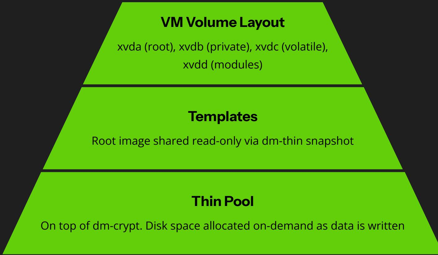
Each qube has its own private storage using LVM thin provisioning, which allocates disk space only as needed. Instead of each AppVM having a full OS copy, they share a base template. Your AppVMs use the same OS image, with VM-specific changes stored in a Copy-on-Write layer on a separate volume.
