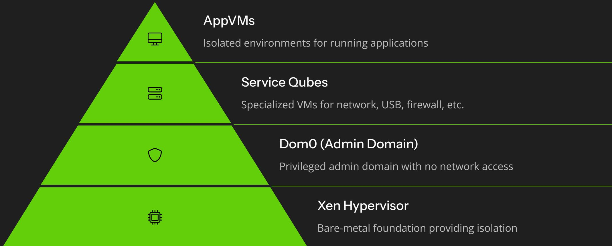
At the core sits the Xen hypervisor, a small layer of code running directly on hardware that allows multiple VMs to run concurrently. Dom0 is the privileged domain controlling all other qubes, while AppVMs run user applications in isolation. Service qubes handle specific functions like networking (sys-net), firewall (sys-firewall), and USB devices (sys-usb).
